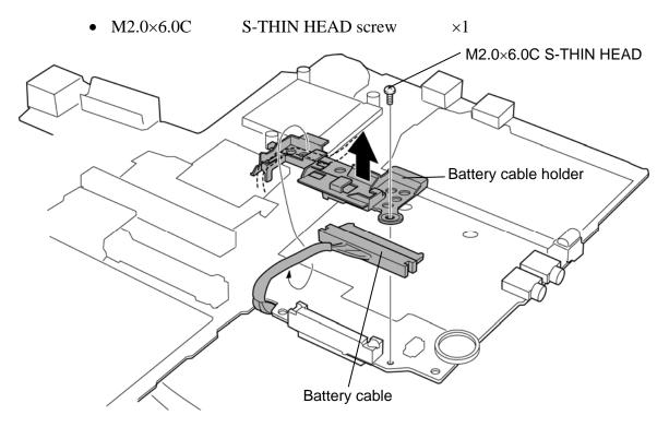
*Figure 4-41 Removing the battery cable holder*
